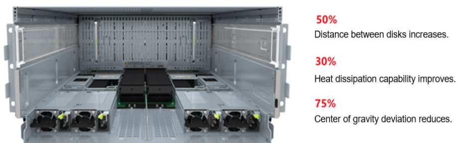
Figure 2-23 Chassis structure of Huawei OceanStor Pacific 9550
